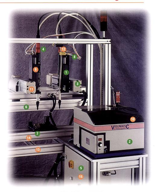
Visumatic develops complete systems to meet your needs. Shown here is a single station to interface with the customer's assembly line, complete with 2 X-Y robots each with a Visumatic VPM-X.2 Power Module. The part is presented to the nosepieces and the screws are stroked into the part with the VPM-X.2 bit stroke module.
